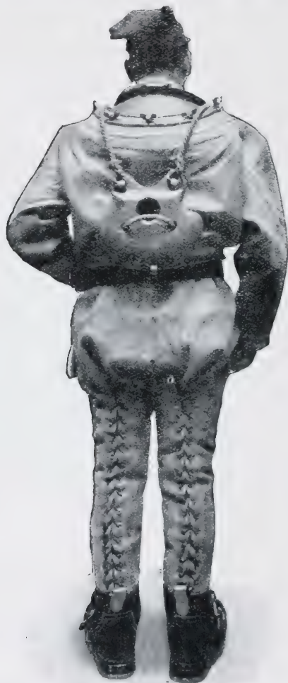
FIG. 24.—DIVING DRESS WITH LEGS LACED UP (SIEBE, GORMAN AND Co.).
